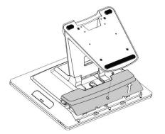
2) Loosen the thumbscrew and slide the stand towards the I/O ports to release from the terminal.
