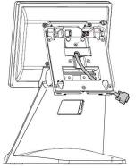
5) Attach the stand to the terminal and secure it with the thumbscrew. Connect the VGA cable to the VGA port on the terminal.
